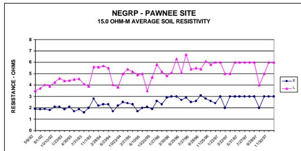
Fig. 3. Resistance graphs of the two most effective electrodes at each site from installation thru end of 1997.
