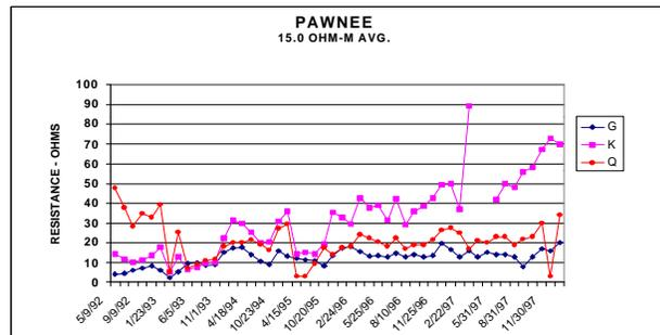
Fig. 4. Resistance graphs of the three least effective electrodes at the Balboa site which has the highest resistivity and the same electrodes at the Pawnee site which has the lowest resistivity.
